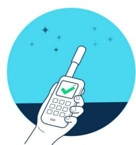
Use your Iridium phone with the antenna extended in an open area where the antenna has an unobstructed 360° view of the sky.
